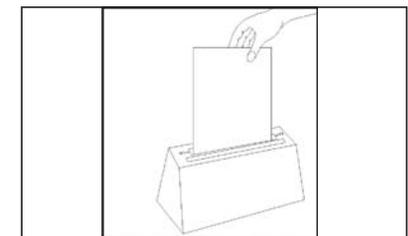
There will be a brief time delay, then the folder will automatically initiate the folding cycle. Once started, the paper should be released.
